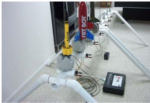
The completed Launch pad and Relay Controller.
